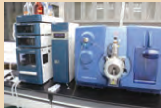
▲中心核心設備—液相層析串聯式質譜儀 Core facility, Liquid chromatograph/ tandem mass spectrometer (LC/MS/MS) in PRAC.
