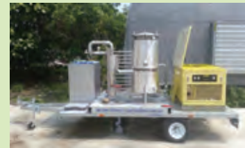
▲ 移動式小型農牧廢棄物氣化發電系統 10 kWe Movable Agriculture and Livestock Waste Gasification Power System/10 kWe
