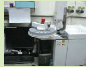
▲微生物脂肪酸鑑定系統 Sherlock™ Microbial Identification System : Fatty Acid Analysis, PLFA & Bacterial ID
